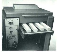
\*Sectional Feed Rolls and Pressure Bar
